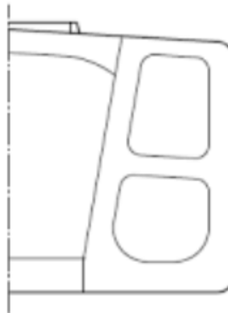
Fig 1 Typical Midship Section of Ore Carriers
