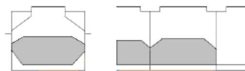
Fig 3 Heavy Cargo Adjacent Holds
